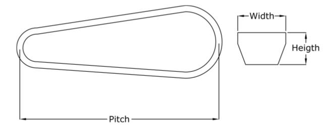
$\begin{array}{ll} \text{Datum Llength} = 8440 \\ \text{Height} &= 12 \\ \text{Length inside} &= 8405 \\ \text{Type} &= \text{CC330} \\ \text{Width} &= 22 \\ \end{array}$
